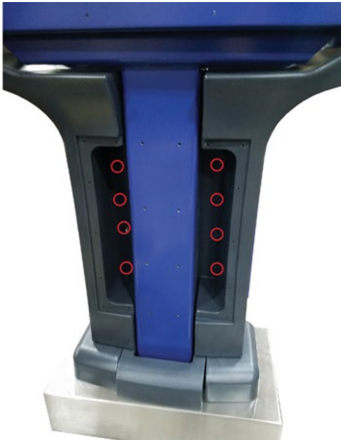
Figure 17. Tighten (8) screws in the rear of the Auto Sentry Petro
