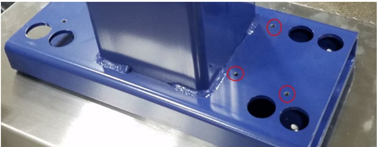
Figure 10. Holes in Metal Base used to Secure Roto Molded parts
