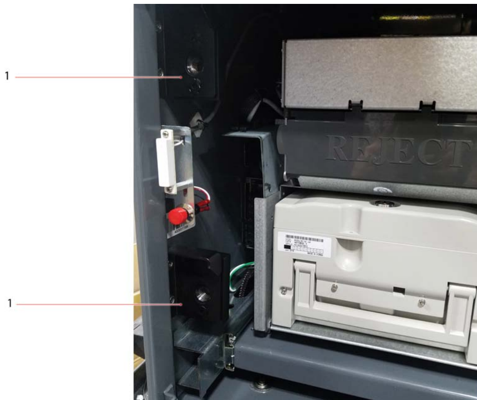
Figure 21. Security Lock Frames, Interior Base
